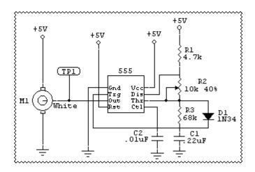
1. Connect the oscilloscope at TP1. Draw the waveform observed and measure the frequency.
