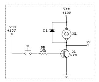
If S1 is open, without measuring, how much base current (I<sub>B</sub>) will flow?
