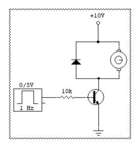
With the frequency of 1 Hz, is the motor on or off?
