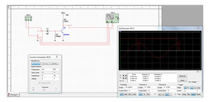
In this lab, we have built the circuit above from the lab manual Figure 31-1. Shown are both input and output waves with the help of Mulitsim. With the square-looking wave as the output, and the sine-wave as the input.
