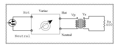
Measure the secondary voltage Vs, which is the voltage across Rs. Use Ohm's law to calculate the current in the load, which is also the current in the secondary winding, Is.
