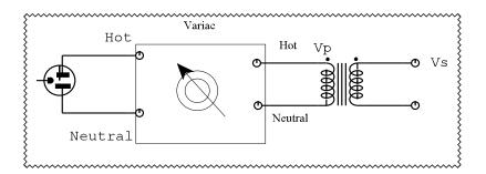
Set the dial of the Variac to the percent setting indicated on the chart. Use a voltmeter to measure the RMS voltage of the Variac output.
